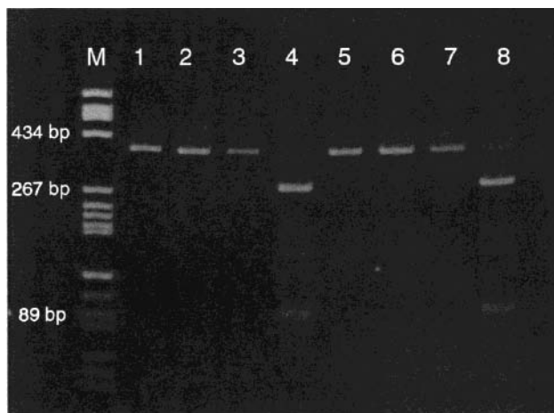
Figure 6. RLFP patterns of Engraulis encrasicolus L. and Sardinella aurita digested with AluI on 7% acrylamide gel, stained with ethidium bromide: (from left to right) molecular weight marker (8÷587 bp) (M); fresh, undigested Engraulis encrasicolus L. (lane 1) and Sardinella aurita (lane 2); fresh, digested Engraulis encrasicolus L. (lane 3) and Sardinella aurita (lane 4); in oil, undigested Engraulis encrasicolus L. (lane 5) and Sardinella aurita (lane 6); in oil, digested Engraulis encrasicolus L. (lane 7) and Sardinella aurita (lane 8).
